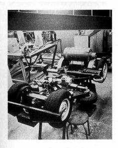
5. The Aramis carcass as it could be seen during the Orly phase. The arms of the on-board steering mechanism allow each cabin to branch off individually; the electric motor will later be replaced by the rotary engine. [Photo RATP]
